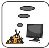
Low Corrosivity IEC60754-2 EN50267-2-2/3 NF C 32-074
