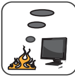
Low Corrosivity IEC60754-2 EN50267-2-2/3 NF C 32-074
